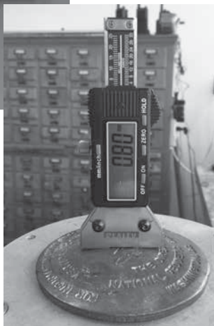
The Digital Depth Gauge, measuring 0.80 mm. Photos courtesy C. Geoghegan.
