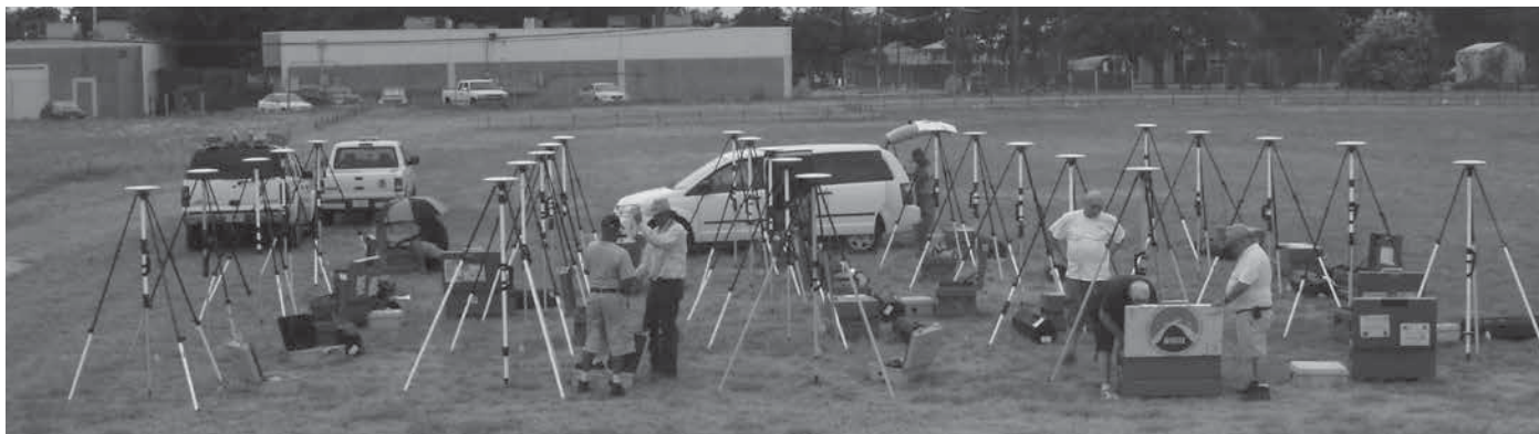
Calibration of the GPS equipment for GSVS11, courtesy C. Geoghegan
