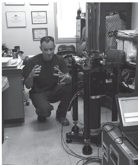
FG5 gravimeter with D. van Westrum explaining how it works. Photos courtesy, P. Fromhertz
